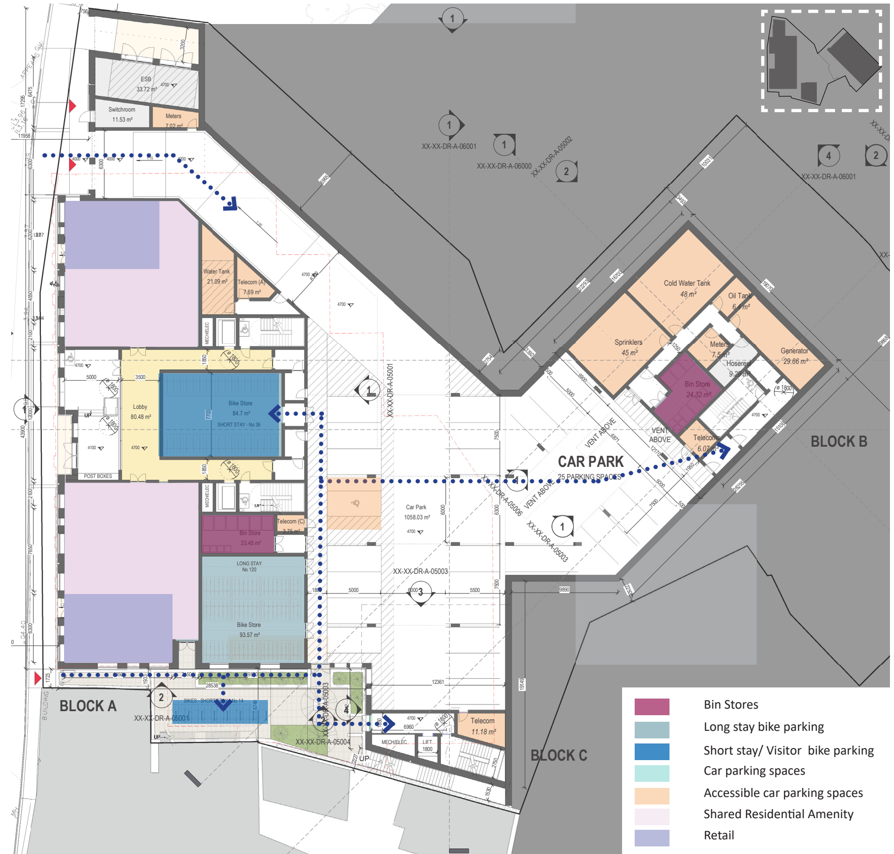
Above: Ground floor diagram describing bike parking locations. Level access is provided to the bike parking from Quay Street and external elevator access is provided from High Street.
